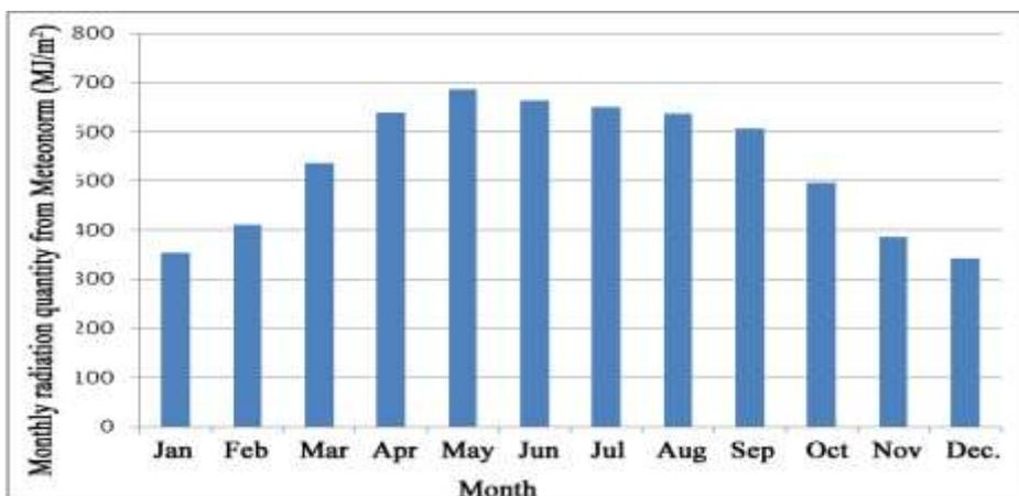
Fig. 2.4 Monthly Average Solar Radiation from Meteonorm (MJ/m<sup>2</sup>)
