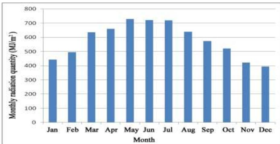
Fig. 2.3 Monthly Average Solar Radiation Quantity in 22 Years from NASA (MJ/m<sup>2</sup>)
