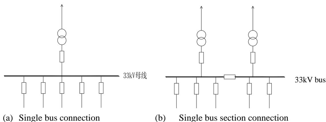
Fig. 3.2 Connection Method for 33kV Switching Station
