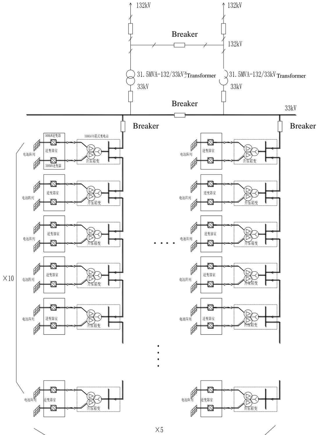
Fig. 3.4 Typical Connection of Power Plant
