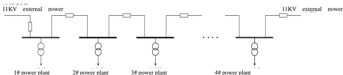
Fig. 3.5 Standby Power Supply Connection Method of the Park
